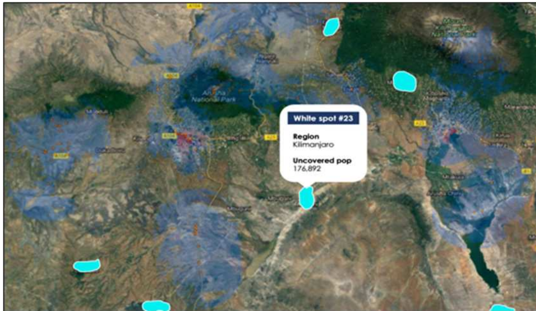
Figure A1.2. Masae Analytics algorithm with granular population density open data and coverage information to detect the most promising zones (“white spots”) for the installation of new base stations
